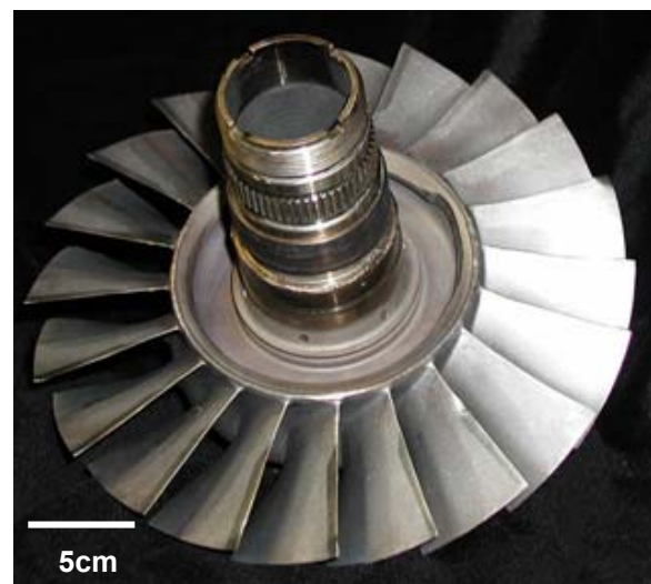
Figure 14. Blisk repair, post finishing, for T700 Engine.
